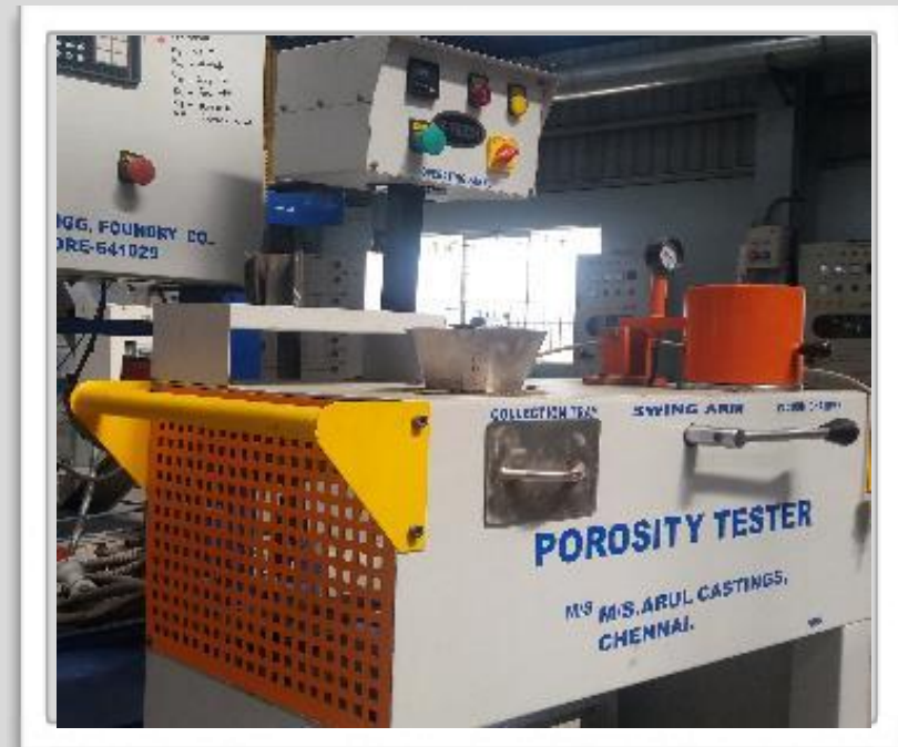
Reduced Pressure Testing
