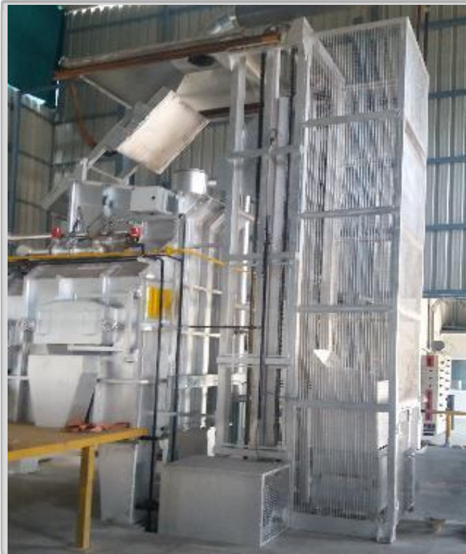
500Kg/hr Tower Furnace Oil Fired.
