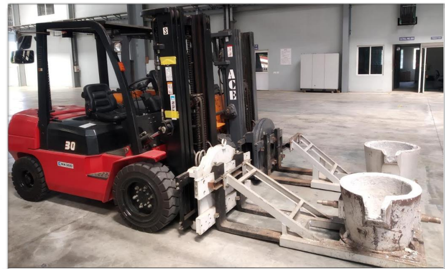
Tiletable swivel type Fork lift -2nos with molten metal transfer ladle
